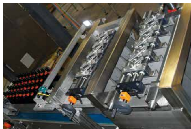
This cutting mechanism is used in the beverage industry. All used components meet the requirement of freedom from lubrication with low weight and low cost.
