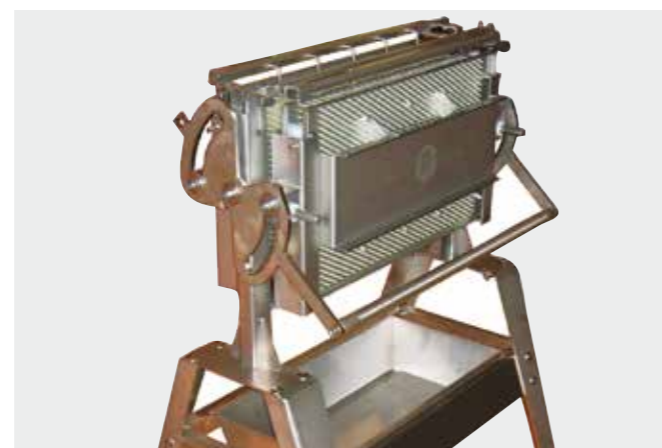
Easy-to-clean and cost-effective iglidur® flanged bearings and clip bearings are used in a honeycomb.
