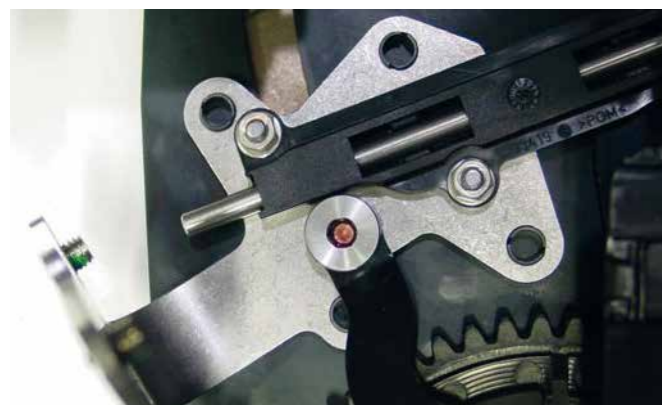
By using wear-resistant iglidur® clip bearings, the lowering mechanism for radiator mascots on luxury cars could be improved.
