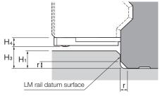
LM Block Side Surface with Side Scrapers Attached
