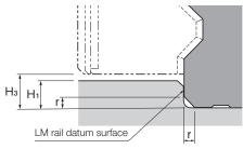
LM Block Side Surface with Protectors Attached
