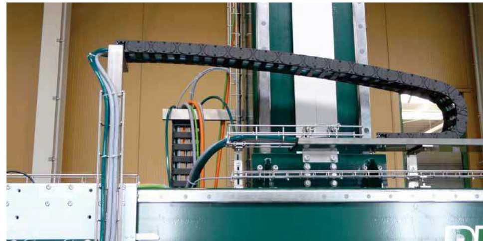
Low weight combined with high strength for long unsupported lengths: E4.1L
