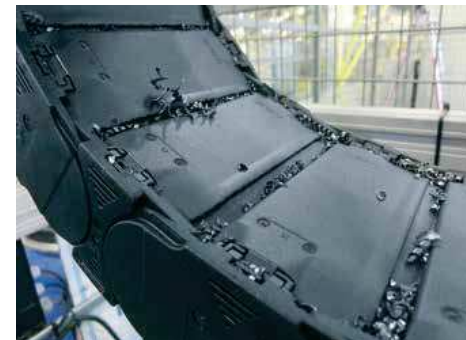
Swarf test in the igus® lab - protection demonstrated in this test setup; stop-dogs completely free of swarf
