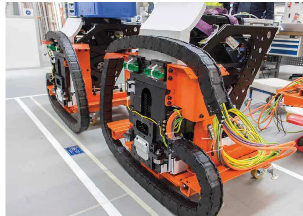
R4.1L e-tubes to guide motor, encoder and sensor cables on a bending machine
